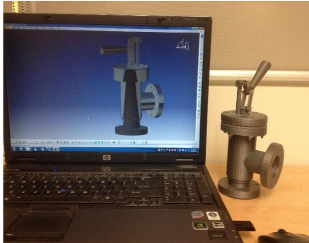
Figure 6: 3D CAD representation and 3D print for a mechanical valve.
